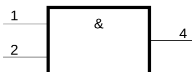
Figure 2. IEC logic symbol
